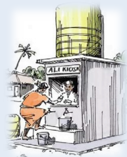
Figure 2.7: Kiosk with storage tank
